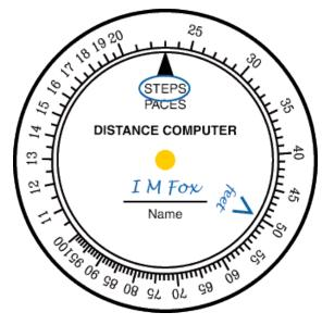
• To find the length of your step, rotate the computer until the "STEPS" marker points to "100." Now the "feet" marker points to about 22. This means that your step length is about 2.2 feet. One thing the distance computer will not do for you is put the decimal point in the right place. You have to do that so the answer makes sense. In this case, the step has to be about 2 feet; 22 feet would be much too big.
