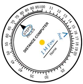
• Now, suppose that we want to step off a distance of 250 feet. To find the number of steps this will take, rotate the computer so that the "feet" marker points to 25. Now the STEPS marker points to 11.5, so we know that we have to go 115 steps.
